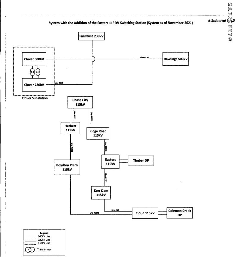
All referenced boxes are substations, with the exception of Cloud Switching Station and Easters Switching Station. All 115kV lines are double circuit lines.
